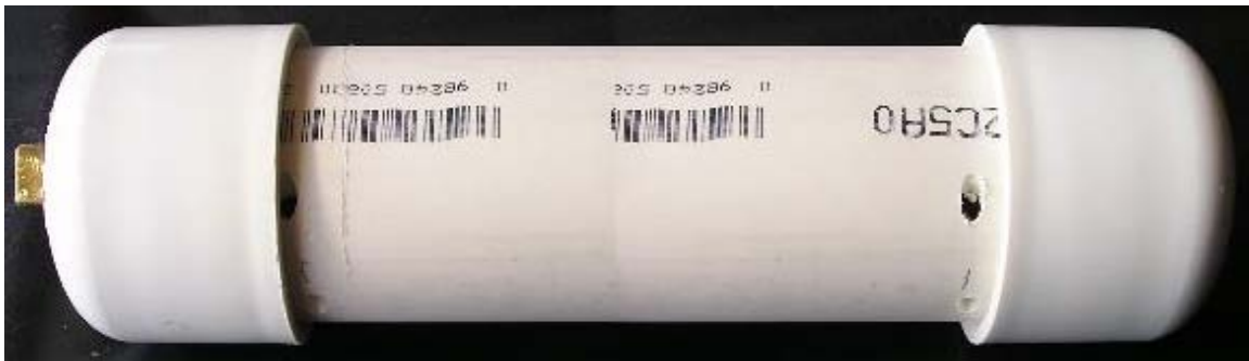
Figure 1: Floatation device constructed from PVC pipe [1]
